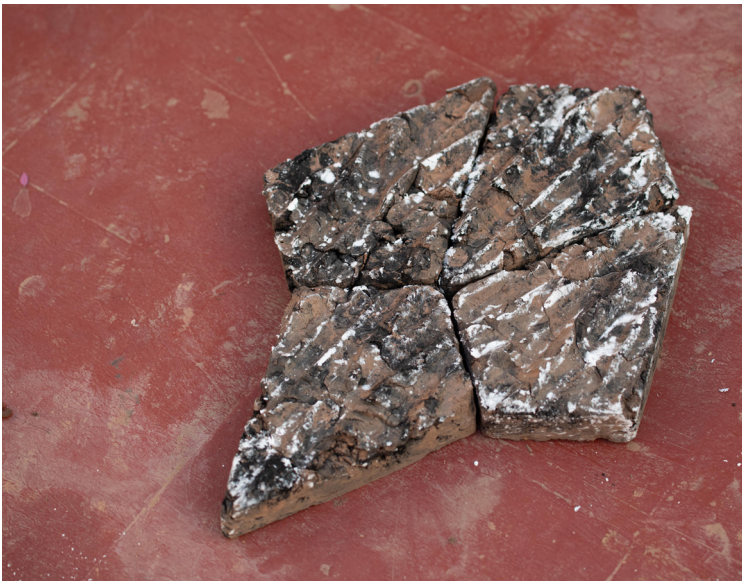
Samples of the tiles that were made with mine waste and clay from Morocco in an ogee shape and a kite shape
