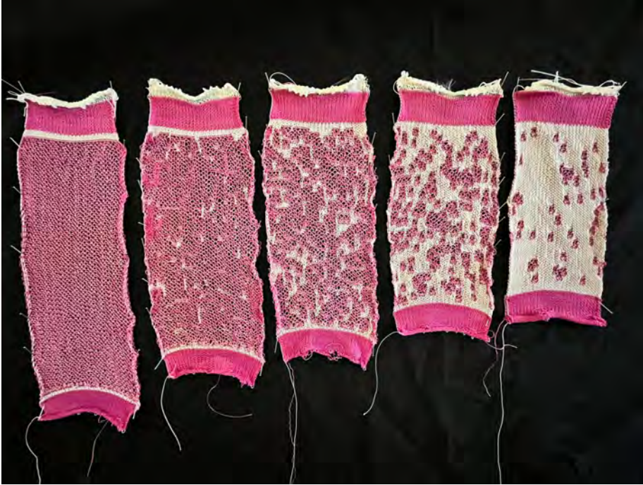
F 5.6: Knitted samples representing five distinct material density gradations used in the GraCe structure. Samples are knitted with Serafil yarn
