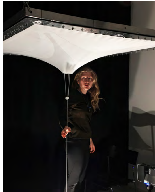
F 3.21: KnitVault tension testing rig. Sinke 2019
