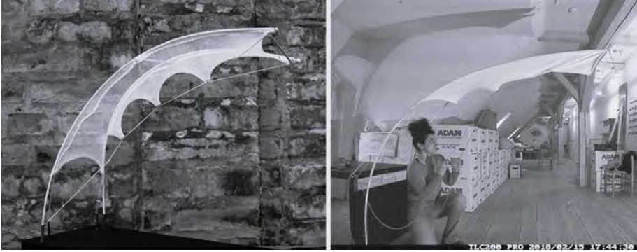
F 1.11: Challenge of knit prediction, specification and the scale up demonstrates the radical difference between the scaled model (to the left) and the 1:1 scale prototype, knitted with the stiff Dyneema fibers (to the right). The figure showcases the difficulty of achieving the same depth of the fabric three-dimensionality at large scale in comparison to the small-scale model. Photos from Isoropia project development at CITA 2017. Photos by Sinke 2017
