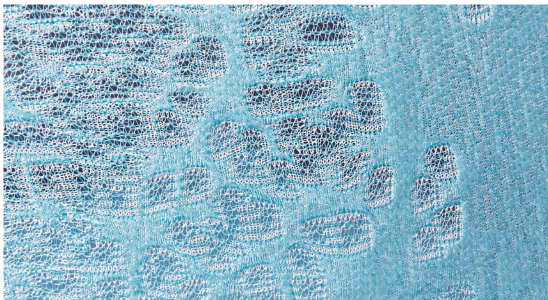
13 Close up of the surface differentiation with the double jacquard and unravel double jacquard stitches
