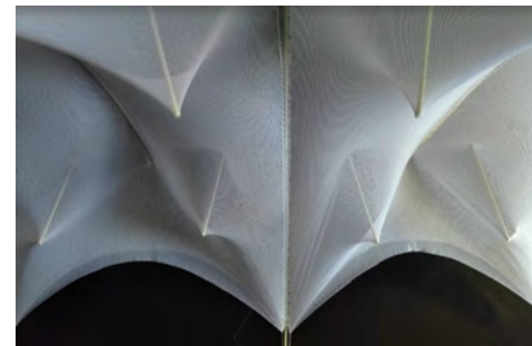
F 3.3: Physical model made of lycra fabric for exploration of membrane novel topologies with compression elements. Pre-studies for Isoropia project at CITA. Sinke 2017
