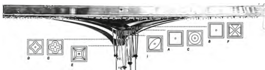
Fig. 4. Side view of 8 samples, performing the difference in depth of the expansion, under load
