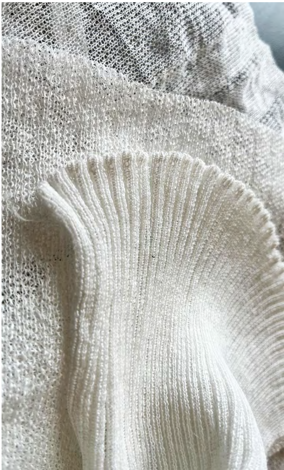
F 5.5: 100% Hemp CNC-knitted samples for RAW research project at CITA 2024, where natural based fibers are investigated for their efficient application in architectural applications. Author of this thesis continues her work with knit in this project. Photo: Y.Sinke
