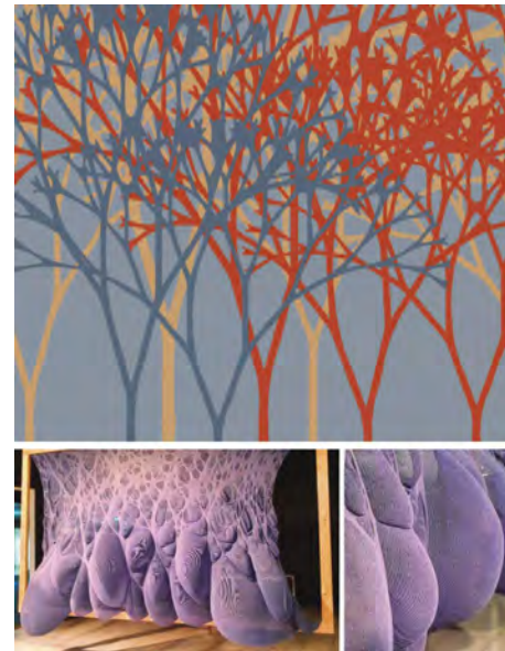
F 2.34: Predefined image knit pattern definition, resulting in volumetric pockets for wind break textiles. Hörteborn and Zboinska 2022
