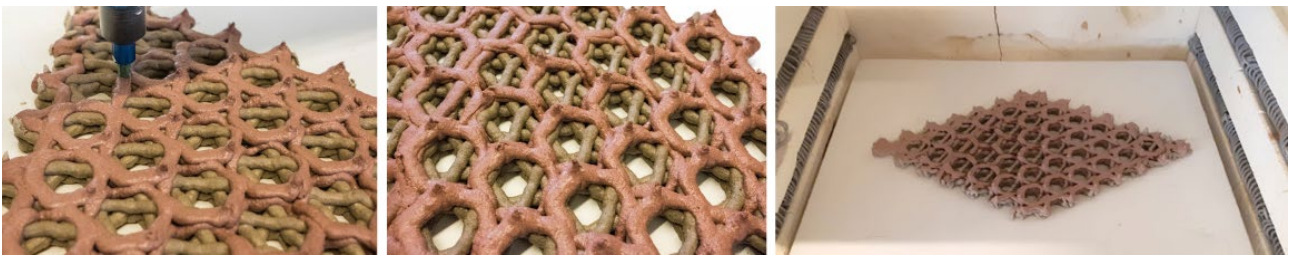
Fig 2: 3D printing process followed by firing
