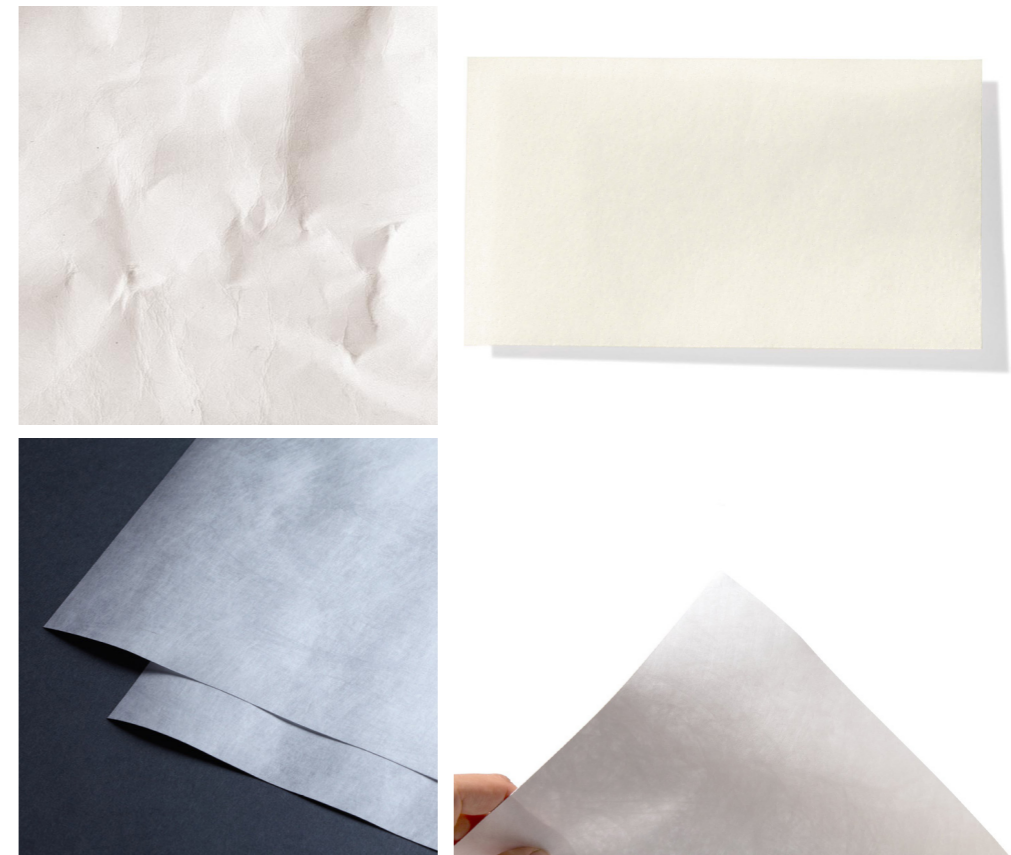
upper left: washable paper; upper right: Modelspan, a tissue paper usually used for airplane models; lower left and right: Tyvek
