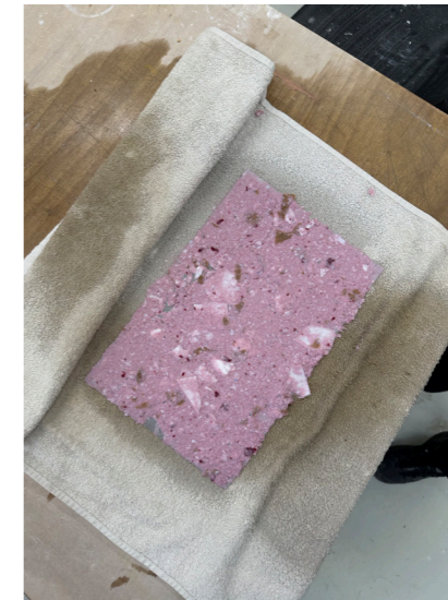
extract a layer of pulp on a flat drain/net and place on towel, drain as much water as possible out and let dry
